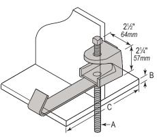
Retainer is supplied flat. Hammer end of retainer up and over beam after clamp is securely attached to beam flange
